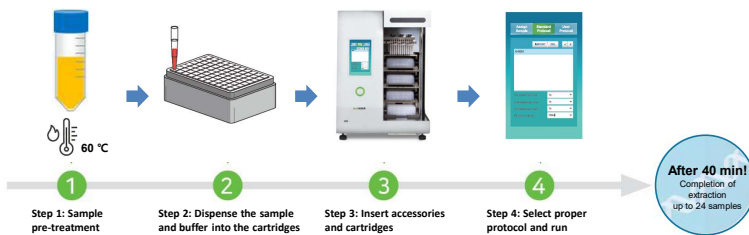
Figure 2. ExiPrep TM 96 Lite cfDNA extraction work flow.
