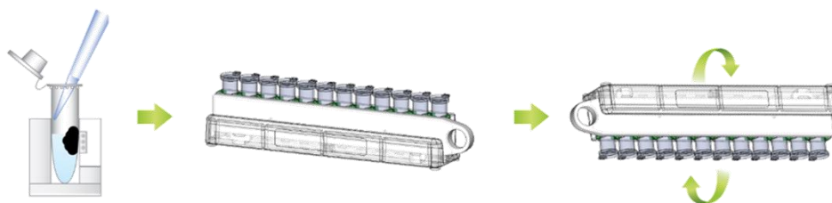
Figure 5. Washing the beads to remove residual ethanol.
