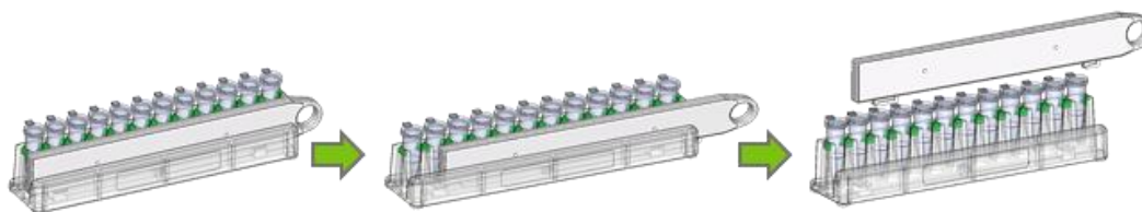
Figure 4. Detachment of the magnet plate. Pull the magnet plate up and gently separate it.
