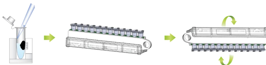
Figure 5. Washing the beads to remove residual ethanol.
