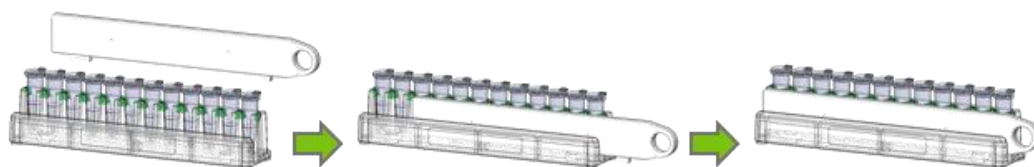
Figure 2. Attachment of the Magnet plate. Combine the magnet plate to the stand.
