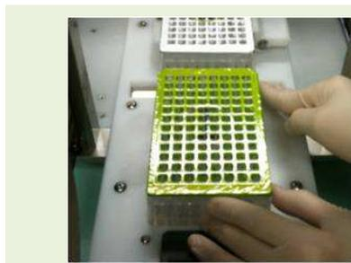
5. Place the Buffer Cartridge ① onto the proper position of the baseplate.
