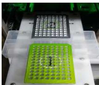
8. Place the Waste tray between Buffer Cartridge ① and ②.
