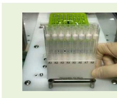
7. Place the Disposable Filter Tip Rack onto the proper position of the base plate.
