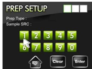
12. The PREP SETUP screen appears as shown in the left, and a screen to select the protocol number for each kit appears. Press '**204**' or '**205**' according to sample type. Confirm following information displayed on the screen, and then press the 'Enter' button.
