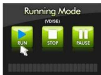
16. In the Running Mode screen, ensure that the protocol name appears on the screen.
