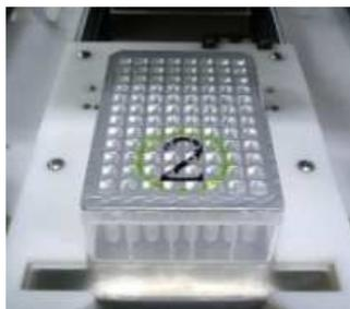
4. Place the Buffer Cartridge ② onto the proper position of the baseplate.
