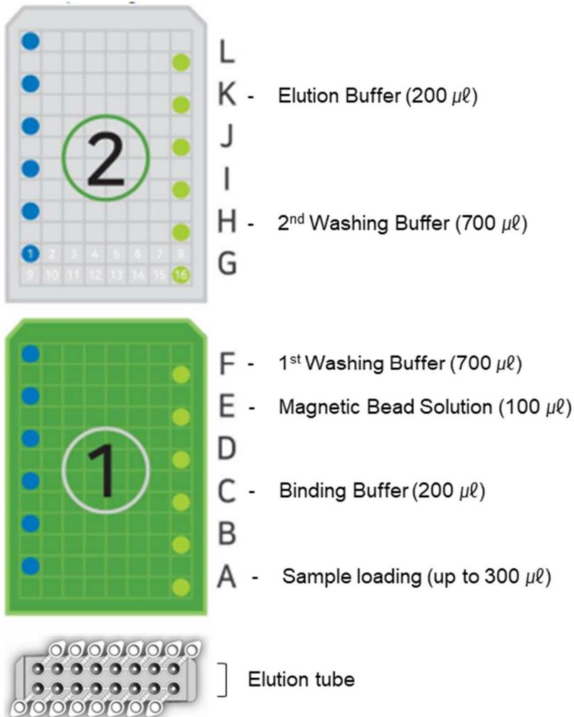
Figure 1. Position of reagents, tubes, and starting material in Cartridges/Elution Tube Rack of ExiPrep™ Plus Plant Total RNA Kit (K-4244).
