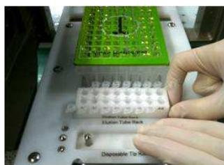
6. Place the Elution Tube Rack including Elution Tubes onto the proper position of the baseplate. The Elution Tube Rack is slotted so it can only be placed in the correct orientation.
