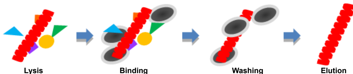
Figure 1. Nucleic acid extraction using silica-coated magnetic nanobeads.
