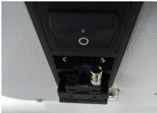
Figure 61. Taking out a fuse from the slot which is disconnected
