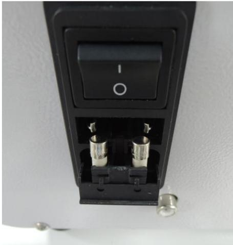
Figure 60. 2 fuses which are inserted
