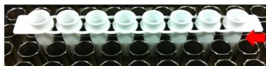
Incorrectly located strip tube
