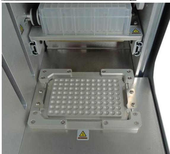
15) Insert elution cartridge into elution heating block.
