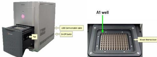
Fig 4. Door-open status of *Exicycler*™ 96 and 96-well thermal block
